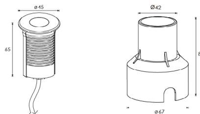
Die-casting grey powder coated aluminum, frame stainless steel.
