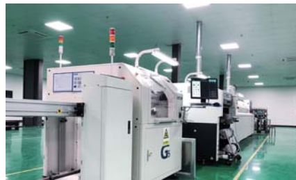
2. Screen Printing Auto Screen Printer: Solder Paste printed to PCB automatically.
